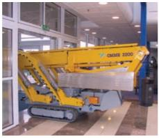
With a width of 1.10m, the Omme 2200 RBD fitted through the narrow entrance and didn't occupy much floor space. Non-marking tracks were needed on the restaurant's finished floor.
